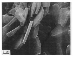
**Figure 1**.- SEM photo of clinoptilolite lamellar crystals of Greek zeolitis.
